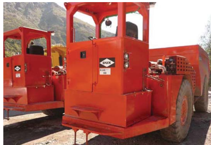
Available with optional bolted spacers for raising FOPS/ROPS operator compartment for improved visibility in reverse.
