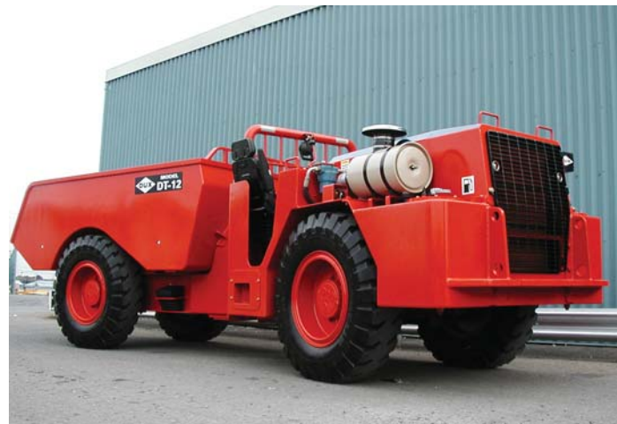
DUX DT-12 with operator compartment located behind front tires.
